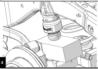
Align the extension on the factory pad with the "shelf" towards the front of the vehicle. Install the provided bolts with washers into the two holes. Torque to 25 ft-lbs.
