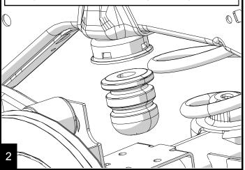
Apply grease to the bumpstop and the extension. Or just the strike pad.
