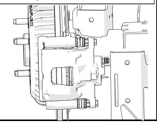
Install the wheel, torque to 110 ft-lbs and repeat these instructions for the other side. Remove the vehicle from the jack stands and place on the ground. Pump the brakes before driving to ensure that the pads are seated firmly against the rotors.
