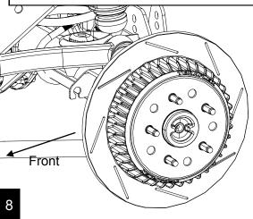
Transfer the pad support springs from the factory caliper bracket to the Teraflex caliper bracket. Apply brake grease everywhere the pads contact the bracket to avoid squeeking.
