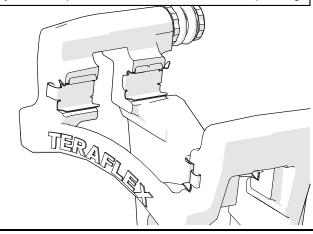
Install the Teraflex bracket onto the vehicle using the factory bolts and a thread locking compound. Torque to 70 ft-lbs.
