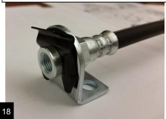
Connect the hard brake lines to the new soft lines and bleed the brakes starting with the passenger side then the drivers side. Note: You will need to purchase shorter metal lines from an auto parts supplier.
