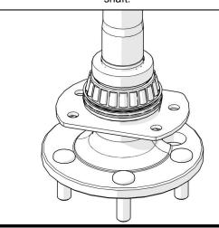
C-clip Axles—Slide the axles all the way into the housing careful not to damage the splines or bearing surface, install c-clips and cross shaft, clean old silicone from the housing and reinstall the differential cover with new gasket or silicone. Refill housing with new oil. C-clips applications proceed to step 16
