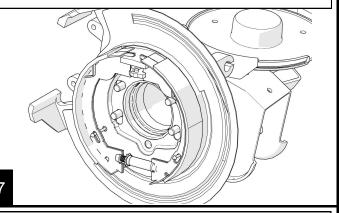
Adjust the internal drum brake with the adjuster until there is just enough room for the rotor to slide over the shoes. This adjustment will set your parking brake tension.
