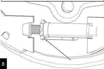
Non– C-clip applications– Install the retaining plate and preload spacer on the axle shaft. **Note: the orientation of the preload spacer is axle dependent.**
