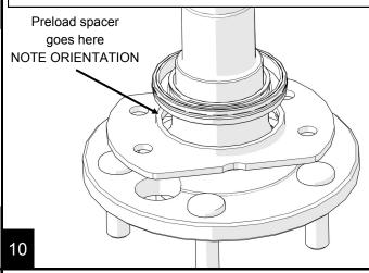
Press the new bearing and retaining collar onto the axle shaft.
