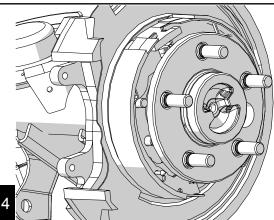
Install and tighten the nuts onto the retainer bolts through the access holes in the axle shaft and install the brake rotor.
