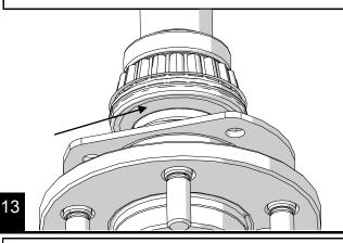
Push the axle in by hand, DO NOT force the axle, seal, splines and/or bearing damage may result.
