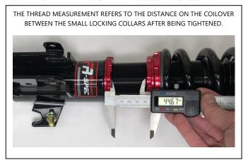
DO NOT GO OUTSIDE THE MAXIMUM AND MINIMUM RANGE DUE TO THE RISK OF DAMAGE TO THE COILOVERS, AXLES, OR OTHER SUSPENSION AND BODY COMPONENTS. ALWAYS CHECK CLEARANCE AFTER INSTALL.
