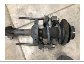
REMOVE TOP HAT, SPRING PERCH, AND SPRING. CLEAN OUT THE LOWER SPRING PERCH ON THE STRUT.
