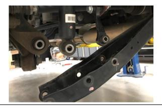
REMOVE REAR TOP HAT NUT AND TOP HAT WITH SPRING COMPRESSORS FOLLOWING SAME PROCEDURE AS FRONT WITH 14mm PASS THROUGH AND 5mm HEX. DISASSEMBLE STRUT.
