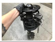
REMOVE TOP HAT NUT WITH 17mm PASS THROUGH AND 6mm HEX KEY. THERE STILL MAY BE SOME PRESSURE, REMOVE WITH CARE. AN OPEN ENDED 17mm WRENCH CAN ALSO WORK HERE.
