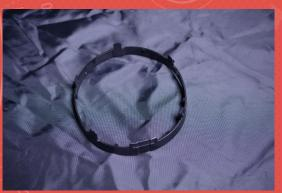
12. FOR 2009-2014 WRX, TURN THE FACTORY BOOT INSIDE OUT AND SEPARATE THE STOCK SHIFT BOOT RING FROM THE BOOT. ONCE SEPERATED, APPLY A THIN LAYER OF ADHESIVE ON THE INSIDE OF THE RING AND INSERT IT INTO AUTOSTYLED BOOT THE SAME WAY IT CAME OUT OF THE FACTORY UNIT. DO NOT OVER-APPLY THE ADHESIVE AS IT CAN BLEED THROUGH THE MATERIAL
