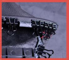
12. ALLOW 10-15 MINUTES FOR THE ADHESIVE TO BOND BEFORE INSTALLING THE BOOT BACK INTO THE VEHICLE. SIMPLY FOLLOW THE REVERSE PROCEDURE TO INSTALL THE NEW AUTOSYTLED BOOT INTO THE VEHICLE
