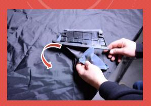
4. USING THE SAND PAPER REMOVE ANY AREAS THAT HAVE FIBER OR ADHESIVE RESIDUE BUILDUP ON THE CORNERS. THIS IS DONE TO ALLOW FOR BETTER ADHESION
