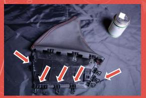
10. REPEAT THE SAME PROCESS ON THE TOP EDGE. REMOVE THE CLIPS, APPLY THE ADHESIVE TO THE CAGE, RESECURE THE CLIPS
