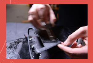
8. ONCE AN EVEN LAYER HAS BEEN APPLIED, SET THE BOOT FIRMLY INTO PLACE. NOTE THAT THE ADHESIVE DRIES QUICKLY SO IT IS VERY IMPORTANT TO MAKE SURE THAT THE PART WAS LINED UP CORRECTLY BEFORE APPLYING ADHESIVE AND SETTING IT IN PLACE
