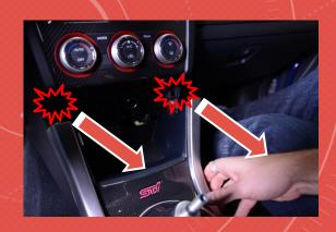
8. SLIDE THE FACTORY SHIFT BOOT OVER THE SHIFTER AND PULL THE ENTIRE ASSEMBLY OUT.
