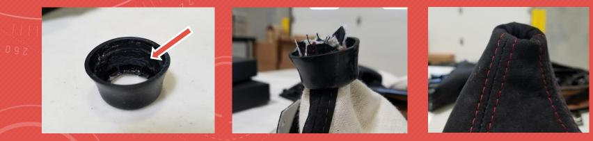
13. TAKING THE AUTOSTYLED SHIFT BOOT, INSTALL IT BACK ONTO THE TRIM SIMILAR TO HOW THE FACTORY UNIT WAS REMOVED. PLEASE NOTE THE SPECIFIC FEATURES ON THE TRIM RING TO ENSURE THE BOOT IS INSTALLED CORRECTLY AS THE BOOT WILL HAVE THE SAME FEATURES
