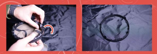
12. FOR 2009-2014 WRX, TURN THE FACTORY BOOT INSIDE OUT AND SEPARATE THE STOCK SHIFT BOOT RING FROM THE BOOT. ONCE SEPERATED, APPLY A THIN LAYER OF ADHESIVE ON THE INSIDE OF THE RING AND INSERT IT INTO AUTOSTYLED BOOT THE SAME WAY IT CAME OUT OF THE FACTORY UNIT. DO NOT OVER-APPLY THE ADHESIVE AS IT CAN BLEED THROUGH THE MATERIAL
