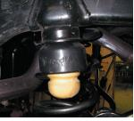
18. Install the lower bump stop onto the axle pad with the 5/16 x 1.25 bolts, washers and nuts provided in the hardware kit. *Note:* Make sure the bumpstop location is the same as photographed with the extra lip facing the front of the vehicle.
