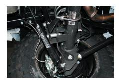
6. Use the provided sleeve as a spacer and install the provided 1/2" by 3.5 bolt through the new bracket and into the factory bracket.
