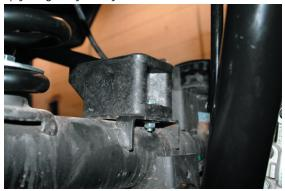
19. To install the rear coil spring retainers on the bottom end of the coil springs first insert the flanged nut into the provided wrench tool, as shown below, and put the nut under the spring pad.
