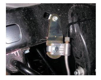
The rear brake line lowering brackets (3-inch kit only. The 4-inch kit includes extended brake and L-Tabs to mount the lines to the frame) are bent in order to allow additional clearance between the brake line and the rear factory sway bar. Be sure to install the left and right brackets so the brake line is moved in away from the sway bar. The locating tab should be located in the slot on the bracket.
