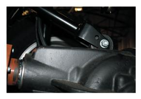
Note: Install the front upper arms as shown in the photo. To avoid removing the exhaust, cut the right front upper control arm bolt on the frame end. A new bolt and nut are included in the kit. Install the new bolt from the outside in. Each lower front FlexArm has a sticker to show where and how to install the arm. Make sure the sticker is up when the arm is installed.
