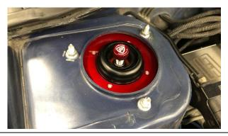
INSERT LOWER MOUNT BOLTS. CAMBER BOLT GOES IN THE TOP HOLE, AND BOTH BOLTS INSERT FROM THE REAR AND POINT TOWARDS THE FRONT OF THE CAR.
