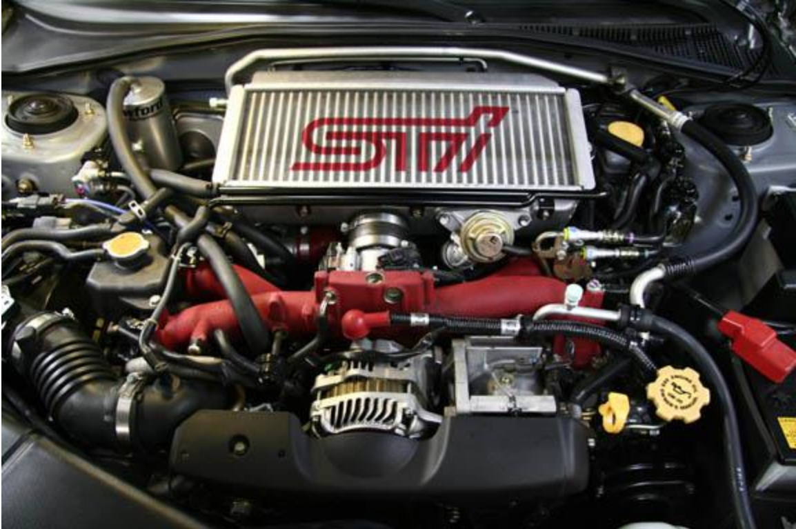
Over view picture of the top mount intercooler air / oil separator location, hoses and mounting point.
