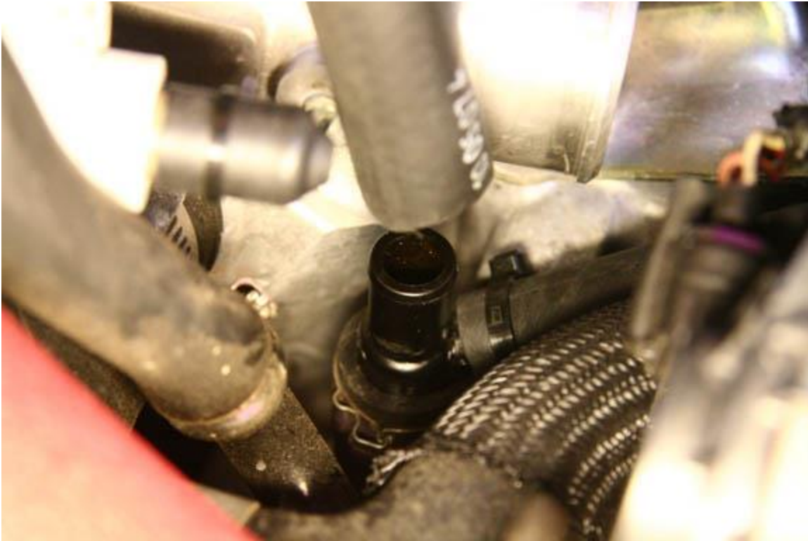
33. Slide the hose over the plastic “Y” connector.
