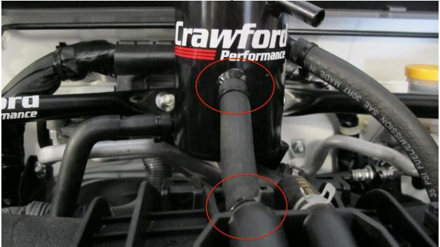
Remove the hose connected to the intake tube before the throttle body and replace it with the 17.5inch hose. Connect it to the top right port of the Air Oil Separator and zip tie both ends.
