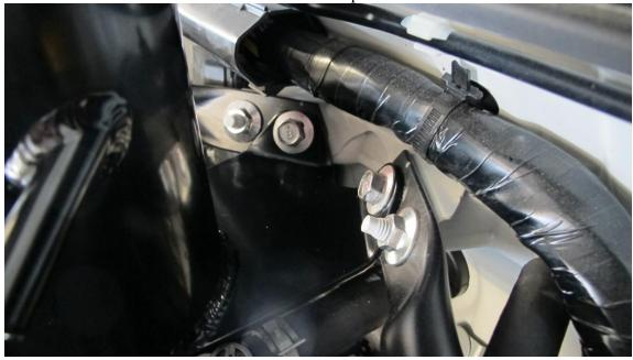
Remove the D-45 cover to expose the hoses and disconnect the PCV hose ONLY from the left port
