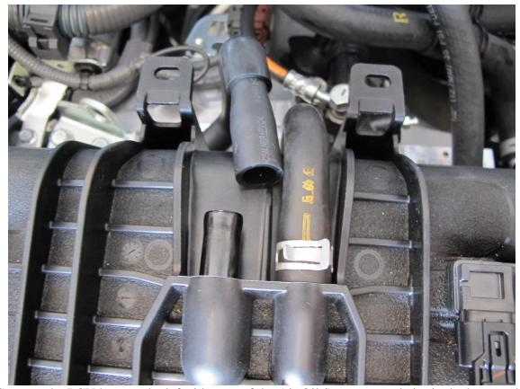
Connect the PCV hose to the left side port of the Air Oil Separator and zip tie the hose to the AOS port
