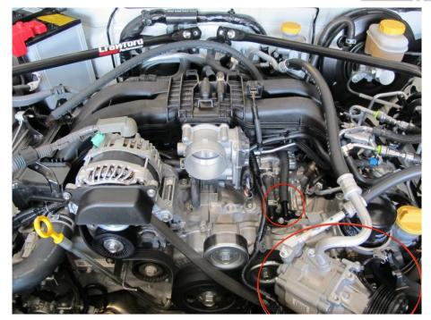
Connect the 19inch hose to the port under the AC pump
