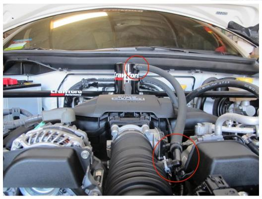
\*\*\* To install the final 19 inch hose you will need to remove the AC pump \*\*\*
