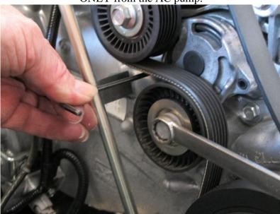
Use a 14mm socket to remove the 3 bolts from the AC bracket (2 front, 1 rear)
