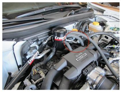
Place the AC pump back in its location and bolt it down to the block. Put the belt back on the AC pump and remove the allen wrench. Allow the tension back into the belt and remove the wrench.
