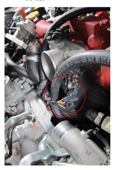
**c.** route hose behind sensor as pictured, either before attaching to the nipple, or by removing and re-attaching the plug
