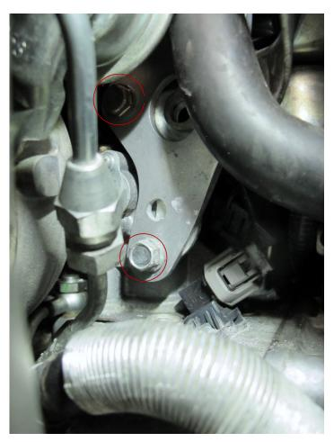
Pictured are the 2 bolts that need to be removed on an STi (aluminum intake manifold)
