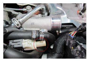
a. Slip worm clamp over hose, and push hose on to nipple until it butts up against sensor
