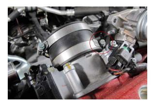
**a.** Loosen screw on the front clamp on throttle body hose. Pull off hose and set aside.
