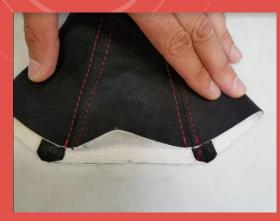
6. REMOVE A FEW CLIPS AND APPLY A THIN LAYER OF ADHESIVE ON THE LOWER PLASTIC TRIM. PLACE THE BOOT BACK IN POSITION AND RE-SECURE THE CLIPS
