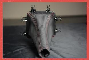
8. USING A PUNCH MAKE A PILOT HOLE IN THE BOOT TO ALLOW THE HARDWARE TO GO THROUGH. ONCE THE PILOT HOLES ARE PLACED, USE A DRILL TO REMOVE ENOUGH MATERIAL ALLOWING THE BOLTS TO BE INSERTED
