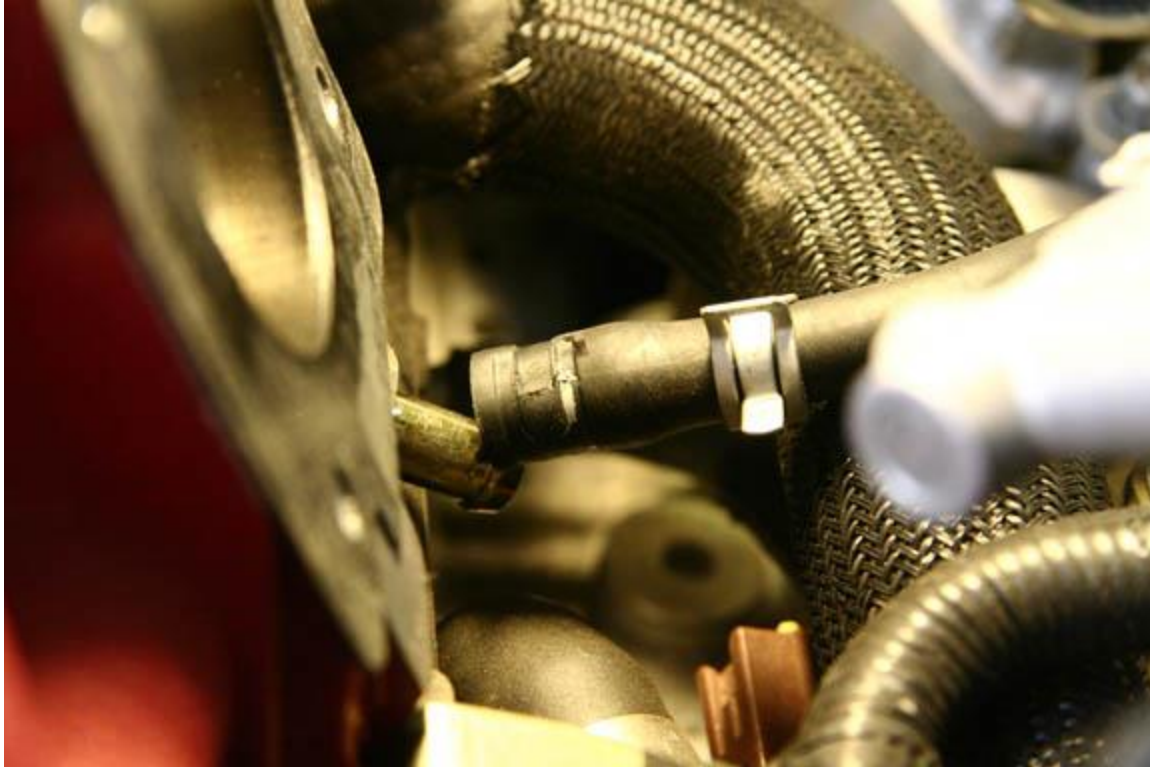
18. Disconnect the rubber hose from the PCV Valve underneath the throttle body.
