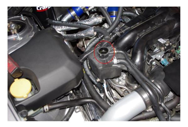
12. Remove the upper coolant line that runs from the expansion tank to the turbo.
