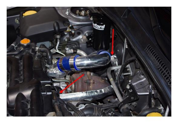
11. Once the car is cool, remove the cap from the coolant expansion tank. You can pinch the lower line running from the expansion tank to the turbo so the coolant doesn't spill. If you lose any coolant, just top it off when finished.
