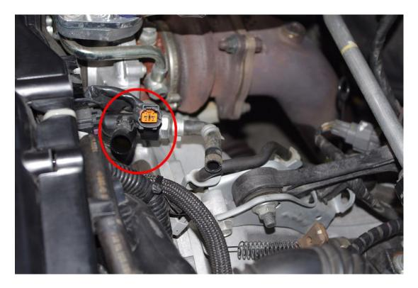
4. Remove the black breather piece from the crankcase breather hose, and remove the smaller black hose from the intake manifold.
