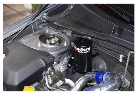
2. Unplug the plug from the white breather piece located behind the intake manifold.
