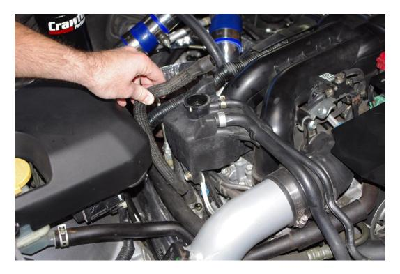
17. Remove the 4" hose that runs from the breather hard line to the driver's side of the intake
