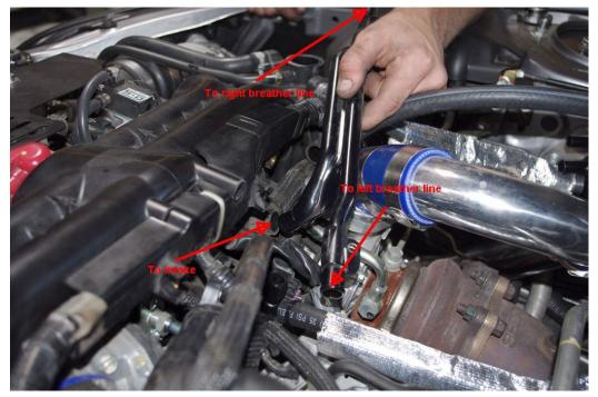
16. Remove the front breather lines (lines closest to the front of the car) from the left and right heads.
