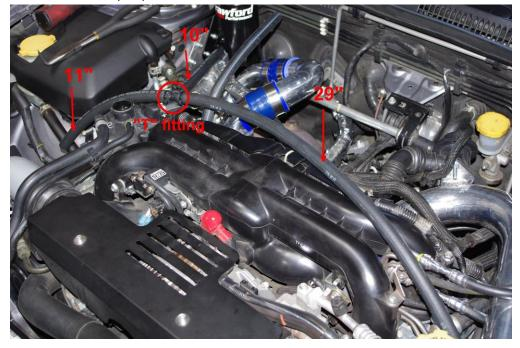
23. Route the 24" long, 5/8" thick hose from the very top of the AOS to the port on the driver's side of the intake (reference step 17 for location). Zip tie to secure.
