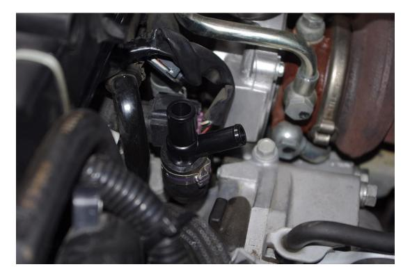
10. Cover the 22" long, ½" wide hose with the 20" fire sleeve. Then route the hose from the very bottom port of the AOS to the bottom of the crankcase breather "Y". Zip tie both ends to secure the hose.
