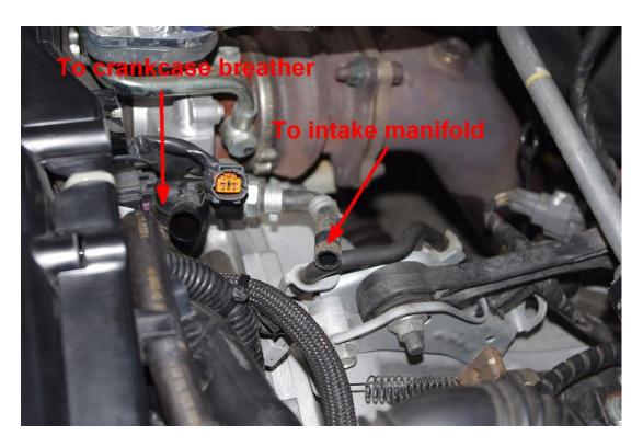
5. Remove the white breather piece from the hose running to the passenger side of the intake, and plug it back into the grey plug. This piece will be a dangler, and can be stowed away after the install is complete.
