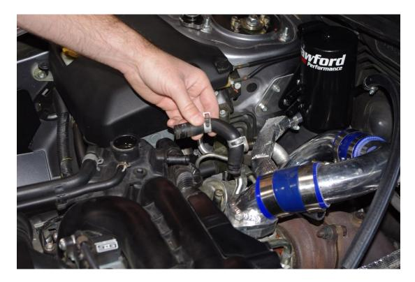
13. Cover the 13.5" heater hose with the 10" fire sleeve, and route it from the front coolant flange on AOS (bottom third port with ribbed edge) to expansion tank. Use supplied clamps to secure.
