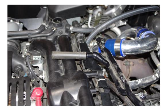
18. Use supplied rubber cap to seal the plastic port on the passenger side of the intake, and zip tie to secure. Large needle nose pliers will make this a bit easier.
