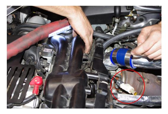
6. Remove the curved rubber hose that runs from the white breather piece to the passenger side of the intake. Here is a photo of it next to the white breather piece for reference (the cap on the breather piece is NOT used)
