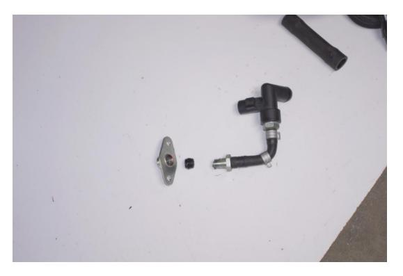
8. Screw the supplied ¼" pipe plug in to the silver metal fitting and replace on the manifold (we lock-tite to keep it secure)
