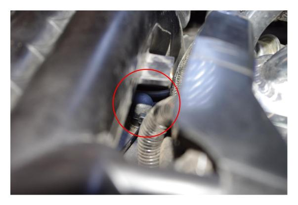
19. Cover the 5/8" thick, 18" long hose with the 10" fire sleeve, and route from the middle port on the AOS to the top of the crankcase breather "Y".
