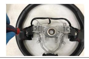
WE ARE READY TO PUT THE OEM COMPONENTS ON THE FACTIONFAB WHEEL. WE RECOMMEND KEEPING THE FOAM ON THE CARBON FIBER WHEELS DURING INSTALL FOR PROTECTION.
