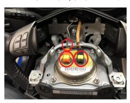
THE MAIN AIRBAG CONNECTORS ARE SIMPLE TO REMOVE. START BY PRYING UP THE YELLOW LOCKING TAB WITH A SMALL FLAT HEAD SCREWDRIVER OR PICK. THE LOCKING TABS COME STRAIGHT UP BUT ARE NOT REMOVED COMLETELY FROM THE CONNECTOR.
