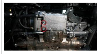
Move the sump to the side. Note that there is a gasket between the sump and the turbo
