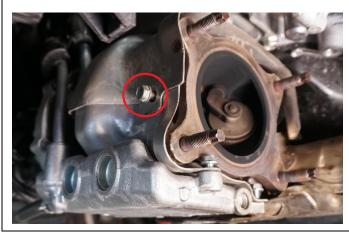
Remove 6 bolts holding the manifold to head. Lower the manifold 2-3" and support in place
