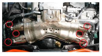
From the back side of the manifold, remove the 2 top heatshield bolts and remove the shield
