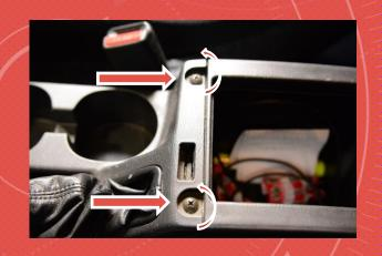
2. EITHER USING A PRY TOOL OR YOUR HAND LIFT THE REAR OF THE SHIFT TRIM. REMOVE THE SHIFT KNOB AND REMOVE THE FACTORY CENTER CONSOLE. ONCE REMOVED UNCLIP THE 12V AND LIGHT FROM THE BACK OF THE TRIM
