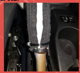
11. TURN THE BOOT BACK RIGHT SIDE OUT AND SECURE IT INTO PLACE, STARTING WITH THE BOTTOM AND WORKING YOUR WAY UP.
