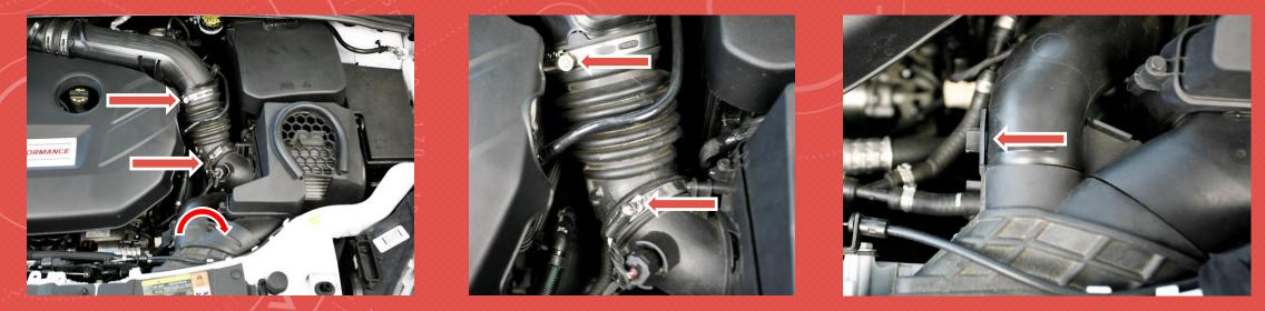
2. PULL UP ON THE AIRBOX EVENLY ON ALL EDGES AND MOVE IT TO THE SIDE ONCE ITS BEEN REMOVED. TAKE A FLAT HEAD SCREWDRIVER AND PRY BETWEEN THE SHIFTER CABLE END AND THE SHIFTER TO DICONNECT THE TWO PIECES IN AN UPWARD DIRECTION
