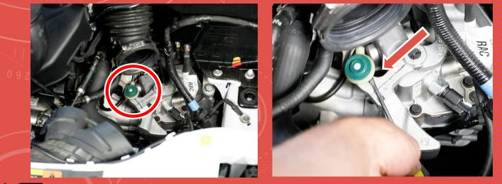
3. DISCONNECT THE TWO SHIFTER CABLES FROM THE SHIFTER BRACKET. THIS IS DONE BY PUSHING ON THE KNURLED SECTION OF THE CABLE AWAY FROM THE BRACKET AND SLIDING THE CABLE OUTWARD.
