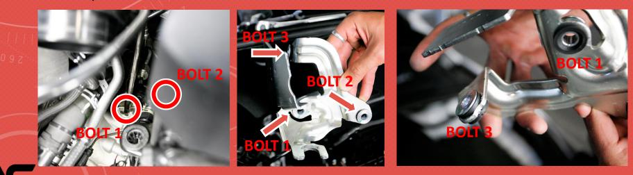
5. NOTE THAT THERE ARE TWO DIFFERENT BOLTS. ONE LONG AND TWO SHORTER. THE LONGER BOLT GOES INTO BOLT LOCATION #2.
