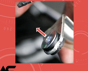
7. APPLY SILICONE/RTV TO THE STEPPED SIDE OF THE NEW AUTOSTYLED BUSHING AND PLACE IT IN THE BRACKET. THIS IS DONE TO KEEP THE BUSHINGS IN PLACE DURING INSTALL. ALLOW FOR THE SILICONE/RTV TO STIFFEN UP FOR 10-30MIN
