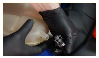
03. Use a cut-up coolant bottle or small container to drain the coolant from the expansion tank. Remove the pressure cap from the tank to expedite the draining process. Some coolant will be pushed out of the small line you disconnected, so be prepared to capture any spills, or use a hose pinch-off tool to clamp the hose.
