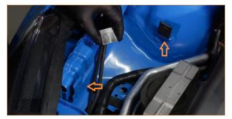
**07.** Remove the isolator from the bottom of the stock expansion tank, and transfer it to the Mishimoto expansion tank.
