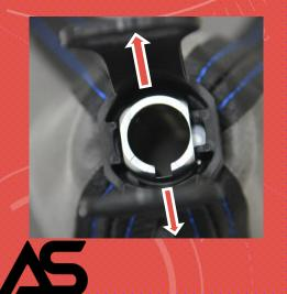
3.3(RS) IF THE CENTER BECOMES DEFORMED DUE TO THE REMOVAL, SIMPLY HEAT IT BACK UP AND USE A SCREWDRIVE TO ROUND IT BACK OUT. BE CAREFUL NOT TO MELT OR DAMAGE THE PART
