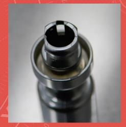
4. REMOVE THE FACTORY BOOT FROM THE CENTER CAGE ALONG WITH ANY REMAINS OF THE STOCK BOOT OR GLUE
