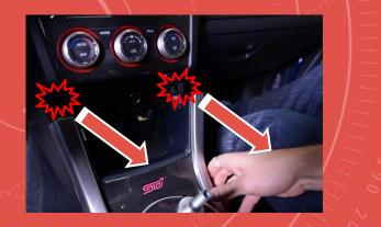
8. SLIDE THE FACTORY SHIFT BOOT OVER THE SHIFTER AND PULL THE ENTIRE ASSEMBLY OUT.
