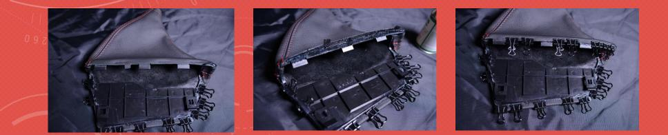
11. WHEN BONDING NEAR THE CLIPS OF THE CAGE THAT SECURE TO THE CENTER CONSOLE, ENSURE THAT THE IS A SLIGHT GAP BETWEEN THE MATERIAL AND THE TOP OF THE CLIP. FAILURE TO DO SO WILL PREVENT THE CAGE FROM SNAPPING INTO PLACE IN THE VEHICLE. IF THERE IS AN ISSUE AFTER INSTALL, SIMPLY REMOVE INTERFERING AMOUNT OF MATERIAL USING A SHARP X-ACTO KNIFE OR RAZOR
