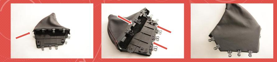
6. ONCE EVERYTHIGN IS 100% IN PLACE AND SECURED. REMOVE THE CLIPS OFF THE <u>LOWER</u> SECTION AND GET READY TO APPLY THE ADHESIVE.
