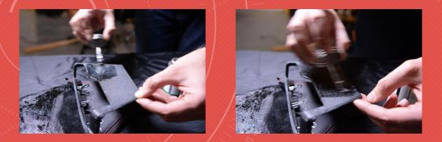
8. ONCE AN EVEN LAYER HAS BEEN APPLIED, SET THE BOOT FIRMLY INTO PLACE. NOTE THAT THE ADHESIVE DRIES QUICKLY SO IT IS VERY IMPORTANT TO MAKE SURE THAT THE PART WAS LINED UP CORRECTLY BEFORE APPLYING ADHESIVE AND SETTING IT IN PLACE
