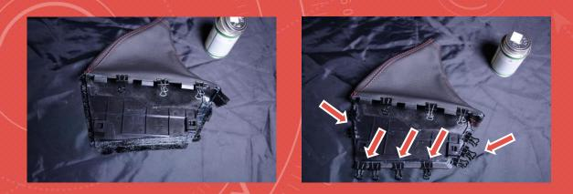
10. REPEAT THE SAME PROCESS ON THE TOP EDGE. REMOVE THE CLIPS, APPLY THE ADHESIVE TO THE CAGE, RE-SECURE THE CLIPS
