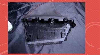
9. APPLY A LAYER OF ADHESIVE ON THE UNDERSIDE OF PLASTIC, TURN THE EDGES OF THE BOOT OVER AND RE-SECURE WITH ALIGATOR CLIPS. WAIT FOR 5-10MIN BEFORE PROCEEDING TO ALLOW TIME FOR THE ADHESIVE TO SET
