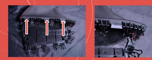
12. ALLOW 10-15 MINUTES FOR THE ADHESIVE TO BOND BEFORE INSTALLING THE BOOT BACK INTO THE VEHICLE. SIMPLY FOLLOW THE REVERSE PROCEDURE TO INSTALL THE NEW AUTOSYTLED BOOT INTO THE VEHICLE
