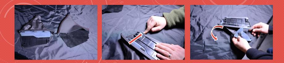
4. USING THE SAND PAPER REMOVE ANY AREAS THAT HAVE FIBER OR ADHESIVE RESIDUE BUILDUP ON THE CORNERS. THIS IS DONE TO ALLOW FOR BETTER ADHESION
