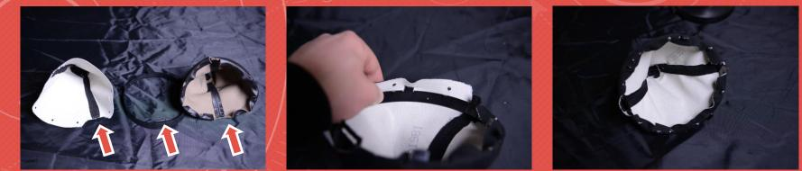
14. WITH THE BOOT INSTALLED ON THE CAGE, SLIDE IT INTO THE SHIFT TRIM BY SECURING THE HORIZONTAL CLIP INTO THE HOUSING FIRST.
