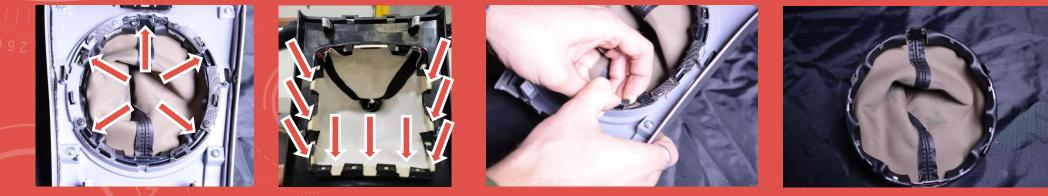
**11. SEPARATE THE FACTORY BOOT FROM THE INTERNAL SUPPORT RING**
