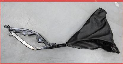
4. INSTALL THE NEW BOOT TO THE CAGE BY APPLYING A LIGHT COAT OF ADHESIVE ONTO THE OUTSIDE LIP IN THE SAME LOCATION AS THE STOCK BOOT. WE FIND IT EASIER TO GLUE ONE SECTION AT A TIME AND START AT THE TOP, WORKING YOUR WAY AROUND. SECURE THE BOOT IN PLACE WITH ALIGATOR CLIPS WHILE YOU WORK ON THE OPPOSITE SIDE.
