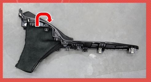
6. SLIDE THE INSIDE-OUT BOOT OVER THE HANDLE UNTIL IT BOTTOMS OUT ON THE HANDLE. THEN USING THE SUPPLIED ZIP-TIE, SECURE THE BOOT TO THE HANLE AND REMOVE THE EXCESS ZIP-TIE WITH DIAGONAL CUTTERS. MAKE SURE THAT THE ZIPTIE GOES INTO THE SLOT/GROOVE AT THE END OF THE HANDLE.
