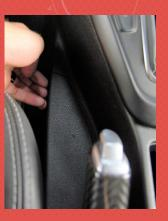
2. USING A SMALL SCREWDRIVER, PRESS ON THE CLIP CENTERS AROUND THE PERIMITER TO SEPARATE THE TWO PIECES
