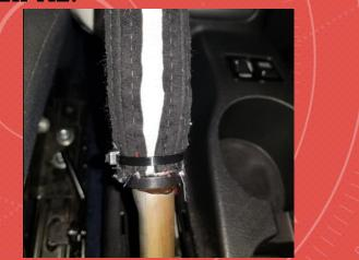
11. TURN THE BOOT BACK RIGHT SIDE OUT AND SECURE IT INTO PLACE, STARTING WITH THE BOTTOM AND WORKING YOUR WAY UP.
