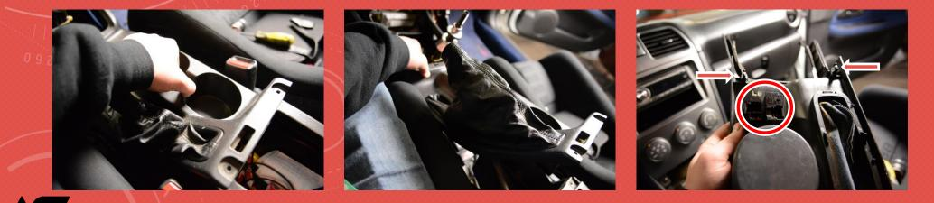
5. PRESS ON THE CLIP AT THE BACK OF SHIFT TRIM AND REMOVE THE FACTORY BOOT AND CAGE
