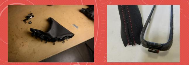
8. ONCE THE BOOT IS POSITIONED REMOVE A FEW CLIPS AND APPLY A LIGHT COAT OF HH-66 ADHESIVE ON THE CAGE. PLACE THE BOOT BACK INTO PLACE ON THE CAGE AND RE-SECURE THE ALIGATOR CLIPS. PROCEED TO DO THIS ALL THE WAY AROUND.
