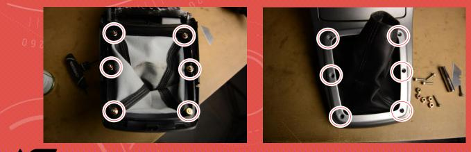
3. SEPARATE THE SHIFT TRIM PIECES BY REMOVING THE TOP RING AND THEN PULLING THE BOTTOM CAGE WITH BOOT OUT
