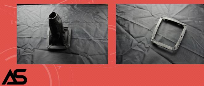
5. PLACE THE AUTOSTYLED BOOT ON THE TRIM AND LINE UP THE CORNERS WHERE THE STITCHES LINE UP OVER THE HOLES. SECURE THE BOOT TO THE BASE USING ALIGATOR CLIPS. NARROW STITCH PATTERN GOES TOWARDS THE REAR
