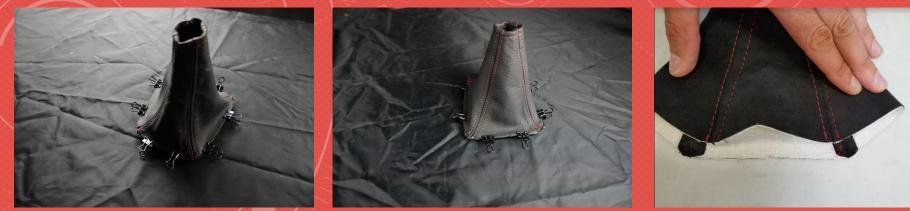
6. REMOVE A FEW CLIPS AND APPLY A THIN LAYER OF ADHESIVE ON THE LOWER PLASTIC TRIM. PLACE THE BOOT BACK IN POSITION AND RE-SECURE THE CLIPS NOTE: DO NOT OVER APPLY THE ADHESIVE AS IT CAN SEEP THROUGH THE MATERIAL.
