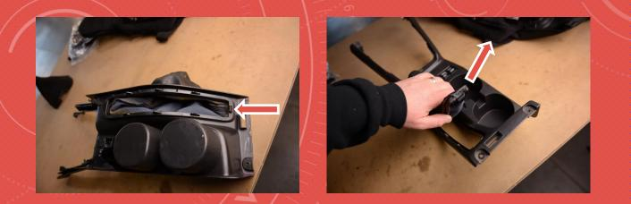
6. SEPERATE THE FACTORY BOOT FROM THE CAGE. NOTE HOW THE BOOT WAS INSTALLED. THIS IS CRITICAL TO NOT INSTALL THE NEW BOOT BACKWARDS
