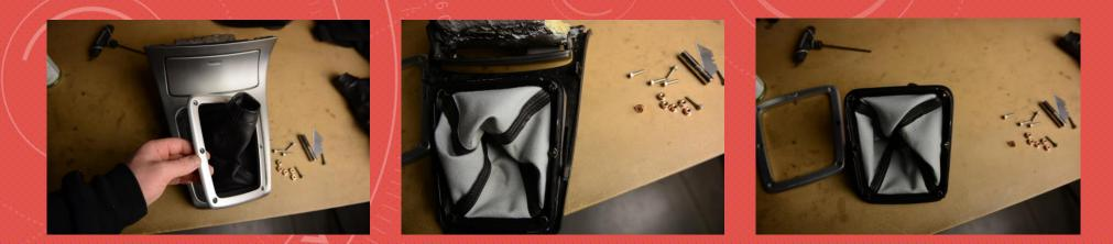
4. SEPARATE THE BOOT FROM THE LOWER PLASTIC CAGE AND REMOVE ANY REMAINING ADHESIVE WITH SAND PAPER
