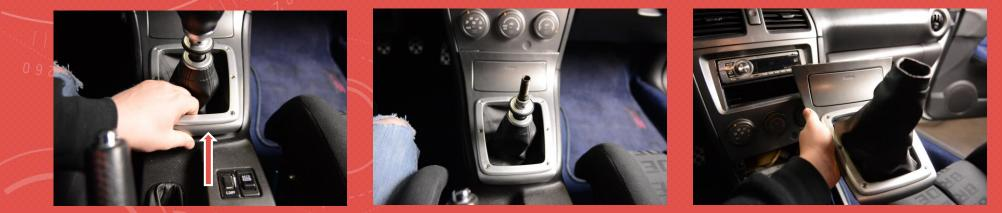
3. REMOVE THE TWO LOWER HEX SCREWS THAT ARE LOCATED ON EACH SIDE OF THE TRIM
