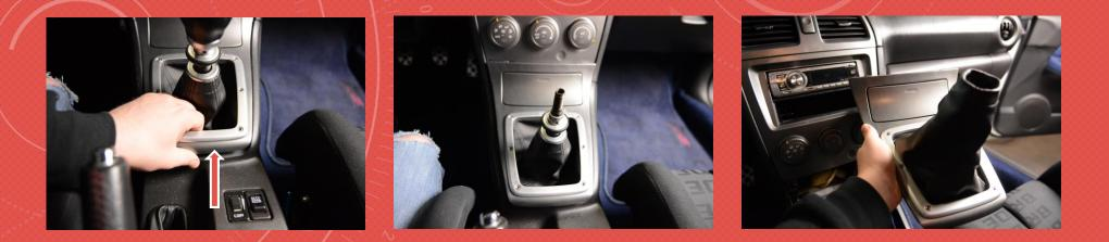
2. USING THE 8MM SOCKET AND 3MM ALLEN, REMOVE THE 6 BOLTS THAT HOLD THE LOWER CAGE TO THE UPPER SHIFT SURROUND
