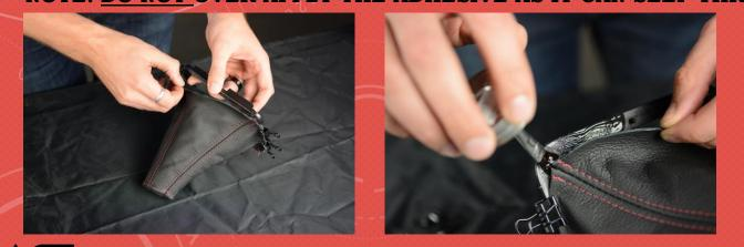
7. REPEAT THE ABOVE STEPS TO SECURE THE REMAINDER OF THE BOOT. ALLOW TO TRY FOR 10MIN BEFORE PROCEEDING
