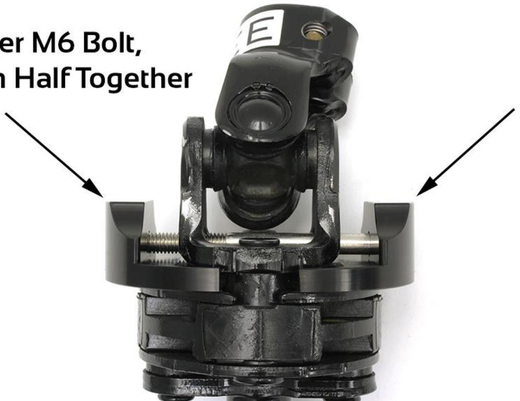
5. Using supplied wrench, slowly tighten bolt compressing both halves together. Once the bolt is tight (both halves should be touching upper half of
