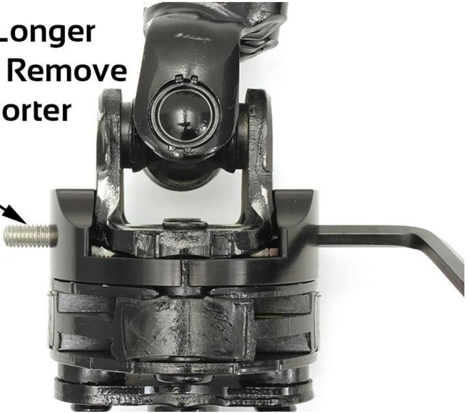
6. Using supplied thread locking compound, apply a few drops to threaded portion of M6x60 bolt.
