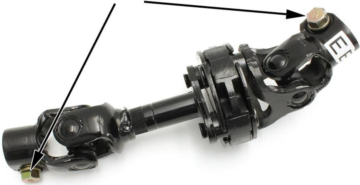
3. Rotate steering wheel until dampener lines up similar to pictures below.
